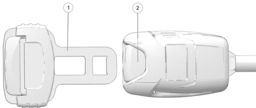
This vehicle is equipped with three-point lap and diagonal seat belts for the operator and any passengers. Always make sure the seat belts are secured for all riders before operating. The driver's seat belt is equipped with a seat belt interlock. Vehicle speed will be limited to 15 MPH (24 km/h) if the seat belt is not secured.
