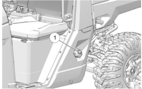
Always ensure that the fuel tank filler cap is fully tightened and secure before operating or transporting the vehicle.
