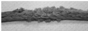
Also replace the winch cable if there are fused or melted fibers. Such an area of the synthetic rope will be stiff and appear smooth or glazed. Promptly discontinue use of a winch cable in this condition.
