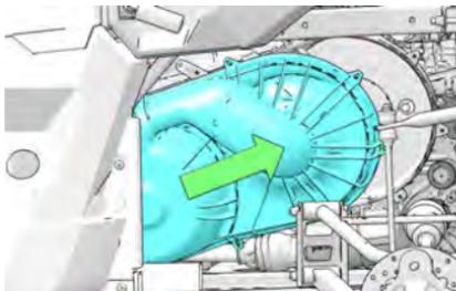
8. Install and torque the outer clutch cover bolts to specification.
