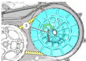
7. Walk the belt out of the driven clutch and drive clutch. Remove the belt from the vehicle.
