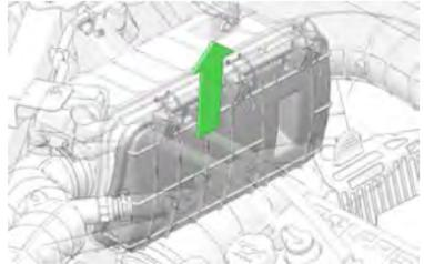
3. Remove the air filter element ①.
