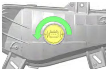
4. Turn the bulb counterclockwise and remove it from the headlight housing, as shown above.
