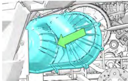
2. Rotate the driven clutch and walk the belt into the clutch.
