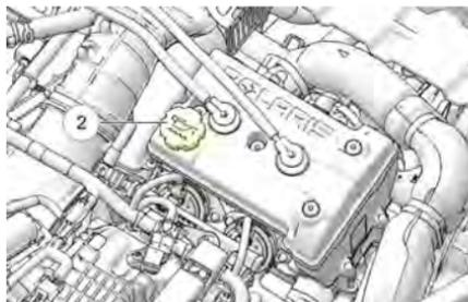
The oil dipstick is located on the engine. Access the dipstick through the right rear wheel well.
