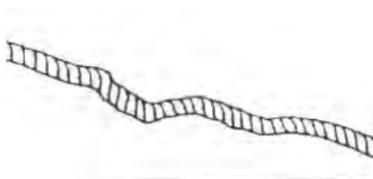
A winch cable made of synthetic rope should be inspected for signs of fraying. Replace the cable if fraying is observed (shown below). Promptly discontinue use of a winch cable in this condition.
