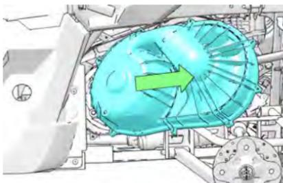
4. Pull clutch cover out towards the rear of the vehicle as shown above.
