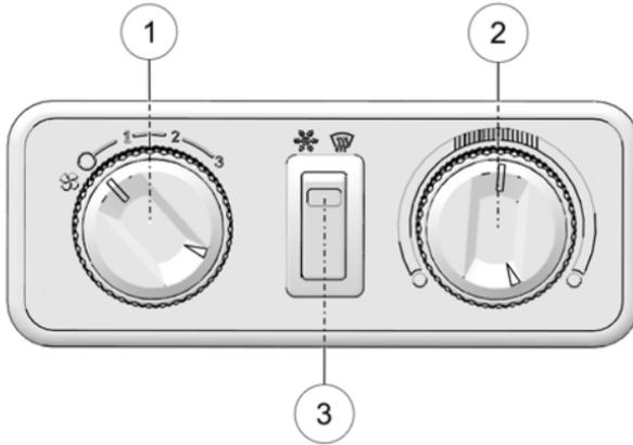
To operate the cab heater, rotate the fan control ① to the desired fan speed setting. The far left setting turns the fan off.
